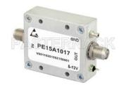
35 dBm IP3, 2 dB NF, 20 dBm P1dB, 500 MHz to 3 GHz, Low Noise Amplifier, 14.5 dB Gain, SMA
