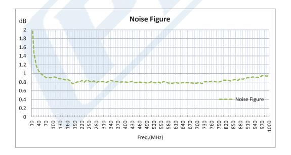
Click the following link (or enter part number in "SEARCH" on website) to obtain additional part information including price, inventory and certifications: 50 dB Gain, 28 dBm IP3, 1 dB NF, 18 dBm P1dB, 10 MHz to 1 GHz, Low Noise High Gain Amplifier SMA PE15A1013
