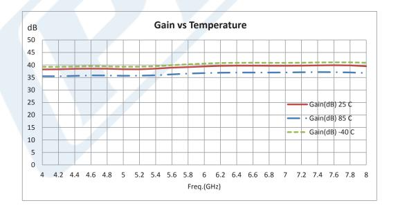
Click the following link (or enter part number in "SEARCH" on website) to obtain additional part information including price, inventory and certifications: 2 dB NF, 20 mW, 4 GHz to 8 GHz, Low Noise Amplifier, 38 dB Gain, SMA PE15A1002
