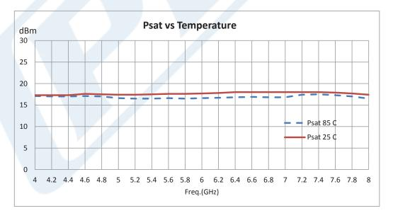
Click the following link (or enter part number in "SEARCH" on website) to obtain additional part information including price, inventory and certifications: 2 dB NF, 20 mW, 4 GHz to 8 GHz, Low Noise Amplifier, 38 dB Gain, SMA PE15A1002
