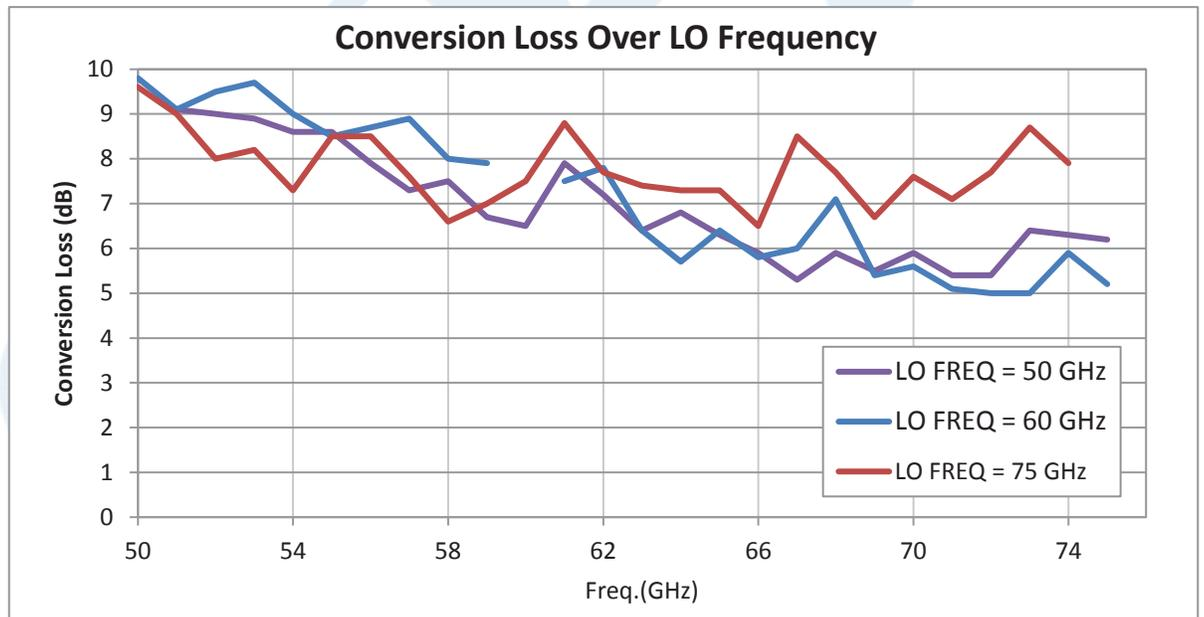
Click the following link (or enter part number in "SEARCH" on website) to obtain additional part information including price, inventory and certifications: [Waveguide Down Converter Mixer WR-15 From 50 GHz to 75 GHz, IF From DC to 18 GHz And LO Power of +13 dBm, UG-385/U Flange, V Band PE12D1002](#)
