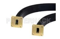
WR-62 Seamless Flexible Waveguide 24 Inch, UG-419/U Square Cover Flange Operating from 12.4 GHz to 18 GHz
