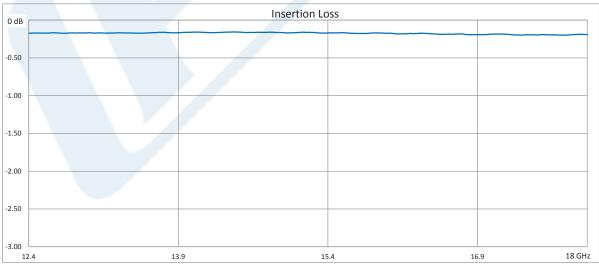
Click the following link (or enter part number in "SEARCH" on website) to obtain additional part information including price, inventory and certifications: WR-62 Seamless Flexible Waveguide 12 Inch, UG-419/U Square Cover Flange Operating from 12.4 GHz to 18 GHz PE-W62SF005-12
