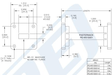
WR-51 Instrumentation Grade Straight Waveguide Section 3 Inch Length with R180 Flange Operating from 15 GHz to 22 GHz from Pasternack Enterprises has same day shipment for domestic and International orders. Our RF, microwave and millimeter wave products maintain a 99% availability and are part of the broadest selection in the industry.
