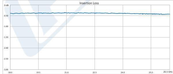
Click the following link (or enter part number in "SEARCH" on website) to obtain additional part information including price, inventory and certifications: WR-42 Seamless Flexible Waveguide 12 Inch, UG-595/U Square Cover Flange Operating from 18 GHz to 26.5 GHz PE-W42SF005-12
