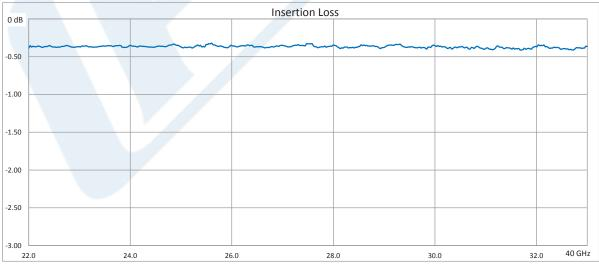
Click the following link (or enter part number in "SEARCH" on website) to obtain additional part information including price, inventory and certifications: WR-34 Seamless Flexible Waveguide 12 Inch, UG-1530/U Square Cover Flange Operating from 22 GHz to 33 GHz PE-W34SF005-12
