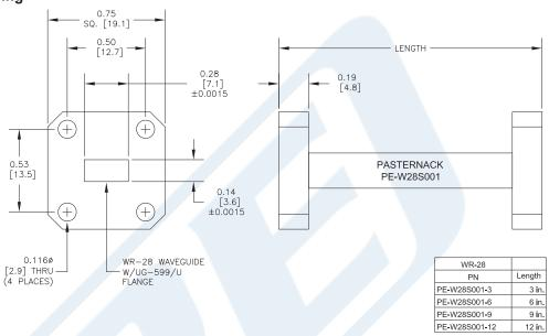
WR-28 Instrumentation Grade Straight Waveguide Section 9 Inch Length with 599/U Flange Operating from 26.5 GHz to 40 GHz from Pasternack Enterprises has same day shipment for domestic and International orders. Our RF, microwave and millimeter wave products maintain a 99% availability and are part of the broadest selection in the industry.
