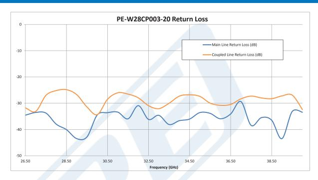
WR-28 Waveguide 20 dB Broadwall Coupler, UG-599/U Square Cover Flange, E-Plane Coupled Port, 26.5 GHz to 40 GHz, Brass Copper from Pasternack Enterprises has same day shipment for domestic and International orders. Our RF, microwave and millimeter wave products maintain a 99.4% availability and are part of the broadest selection in the industry.
