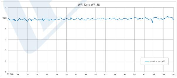
Click the following link (or enter part number in "SEARCH" on website) to obtain additional part information including price, inventory and certifications: WR-22 to WR-28 Waveguide Transition 2 Inch Length, UG-383/U Round Cover Flange to UG-599/U Square Cover Flange PE-W22TS28001
