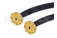
WR-22 Seamless Flexible Waveguide 12 Inch, UG-383/U Round Cover Flange Operating from 33 GHz to 50 GHz
