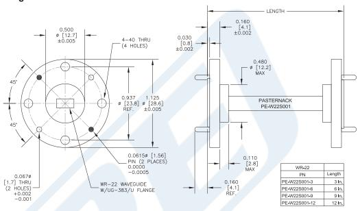
WR-22 Instrumentation Grade Straight Waveguide Section 9 Inch Length with UG-383/U Flange Operating from 33 GHz to 50 GHz from Pasternack Enterprises has same day shipment for domestic and International orders. Our RF, microwave and millimeter wave products maintain a 99% availability and are part of the broadest selection in the industry.
