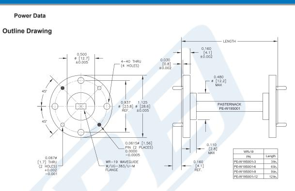
WR-19 Instrumentation Grade Straight Waveguide Section 9 Inch Length with UG383/U-Mod Flange Operating from 40 GHz to 60 GHz from Pasternack Enterprises has same day shipment for domestic and International orders. Our RF, microwave and millimeter wave products maintain a 99% availability and are part of the broadest selection in the industry.
