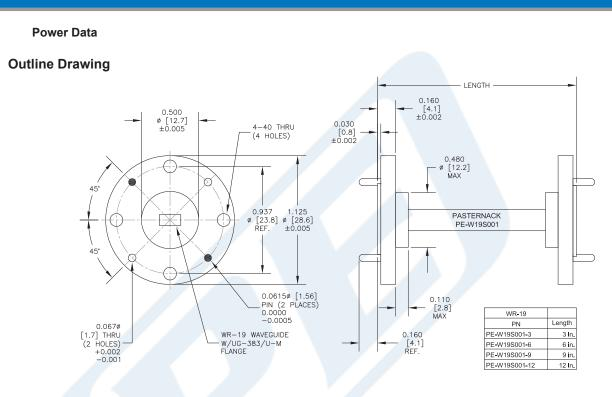
WR-19 Instrumentation Grade Straight Waveguide Section 6 Inch Length with UG383/U-Mod Flange Operating from 40 GHz to 60 GHz from Pasternack Enterprises has same day shipment for domestic and International orders. Our RF, microwave and millimeter wave products maintain a 99% availability and are part of the broadest selection in the industry.
