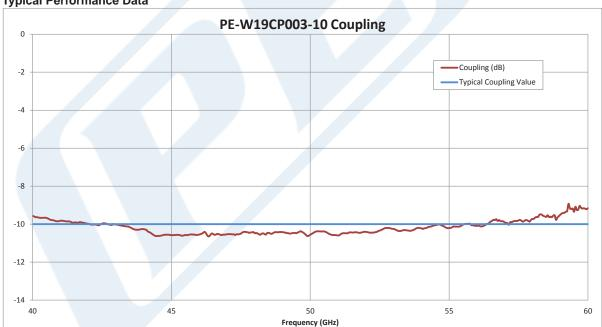
Click the following link (or enter part number in "SEARCH" on website) to obtain additional part information including price, inventory and certifications: WR-19 Waveguide 10 dB Broadwall Coupler, UG-383/U Round Cover Flange, E-Plane Coupled Port, 40 GHz to 60 GHz, Brass Copper PE-W19CP003-10
