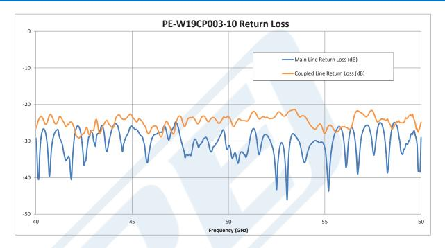
WR-19 Waveguide 10 dB Broadwall Coupler, UG-383/U Round Cover Flange, E-Plane Coupled Port, 40 GHz to 60 GHz, Brass Copper from Pasternack Enterprises has same day shipment for domestic and International orders. Our RF, microwave and millimeter wave products maintain a 99.4% availability and are part of the broadest selection in the industry.
