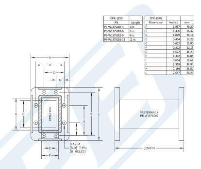
WR-137 Commercial Grade Straight Waveguide Section 9 Inch Length with CPR-137G Flange Operating from 5.85 GHz to 8.2 GHz from Pasternack Enterprises has same day shipment for domestic and International orders. Our RF, microwave and millimeter wave products maintain a 99% availability and are part of the broadest selection in the industry.
