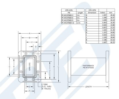
WR-137 Commercial Grade Straight Waveguide Section 3 Inch Length with CPR-137G Flange Operating from 5.85 GHz to 8.2 GHz from Pasternack Enterprises has same day shipment for domestic and International orders. Our RF, microwave and millimeter wave products maintain a 99% availability and are part of the broadest selection in the industry.
