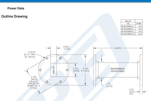
WR-137 Commercial Grade Straight Waveguide Section 6 Inch Length with UG-344/U Flange Operating from 5.85 GHz to 8.2 GHz from Pasternack Enterprises has same day shipment for domestic and International orders. Our RF, microwave and millimeter wave products maintain a 99% availability and are part of the broadest selection in the industry.
