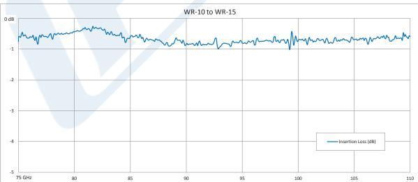
Click the following link (or enter part number in "SEARCH" on website) to obtain additional part information including price, inventory and certifications: WR-10 to WR-15 Waveguide Transition 1.5 Inch Length, UG-387/U-Mod Round Cover Flange to UG-385/U Round Cover Flange PE-W10TS15001
