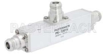
Low Loss 6 dB N Unequal Tapper Optimized For Mobile Networks From 380 MHz to 6 GHz Rated To 300 Watts
